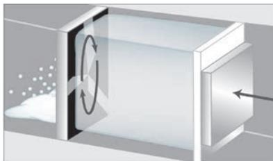
*Cold Jet's patented feeder technology creates shaved dry ice on demand, regardless of input.*
