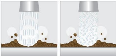
*Simply switch to full pellet cleaning to penetrate the most difficult, thick contaminants.*
